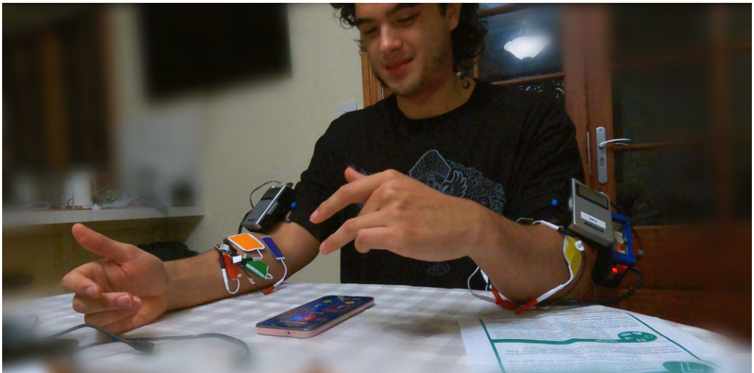
Fig. 12. A participant looks at the phone to confirm their interpretation of the EMS-controlled hand’s resulting gesture.
